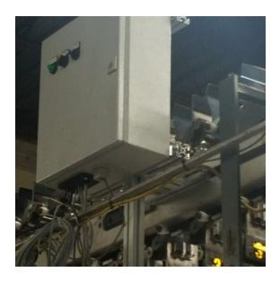
The Printer Control Panel (PCP) manages the signals from the sensors and the printer.
